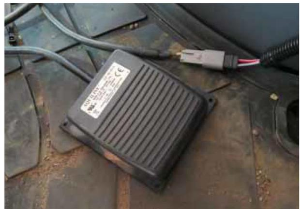
FIGURE 36 RESUME FOOT SWITCH CONNECTION
