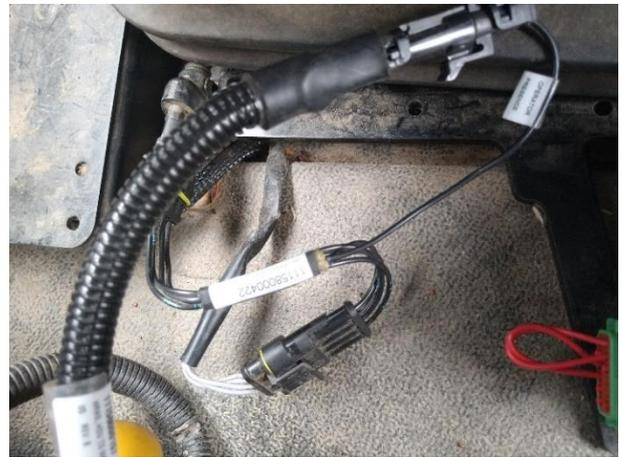
FIGURE 38 OPERATOR PRESENCE SWITCH T-CABLE (115-8000-428) CONNECTION
