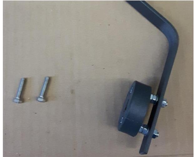
FIGURE 26 WHEEL ANGLE SENSOR DISC MOUNTED WITH SPACERS.
