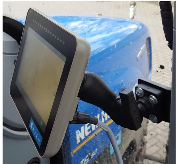
FIGURE 49 RAM-C BALL ATTACHEMENT
