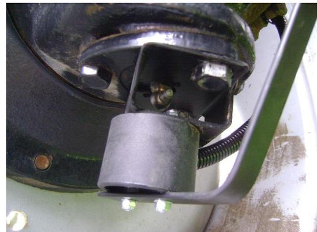
FIGURE 20 STUB AXLE WITH GREASE NIPPLE.
