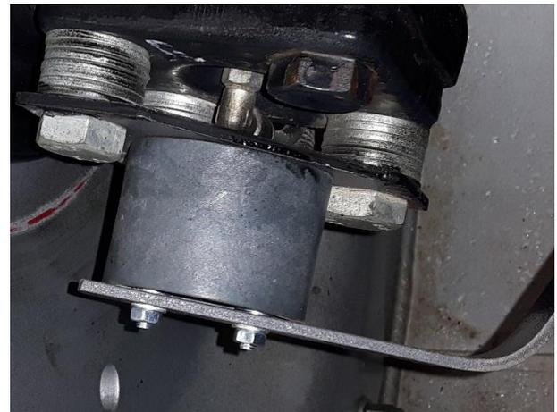
FIGURE 30 CORRECT MOUNTED WHEEL ANGLE SENSOR
