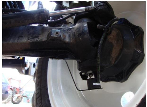
FIGURE 19 STEERING ANGLE SENSOR ON NEW HOLLAND.
