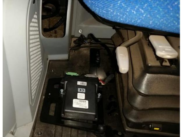
FIGURE 3 A SC1/TC1 MOUNTED NEXT TO THE SEAT
