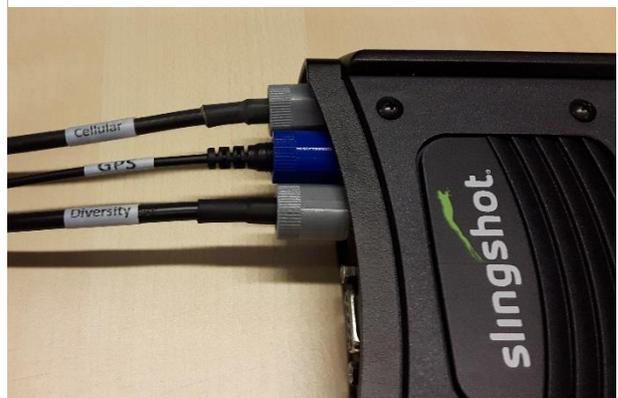
FIGURE 47 ANTENNA CABLES WITH LABELS AND SMA-GRIP SET.
