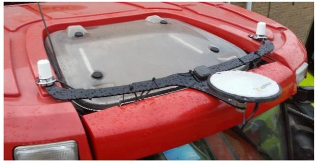
FIGURE 45 CASE NEW HOLLAND WITH GPS-ANTENNA, GPS PATCH ANTENNA AND TWO GPRS/UMTS ANTENNA'S
