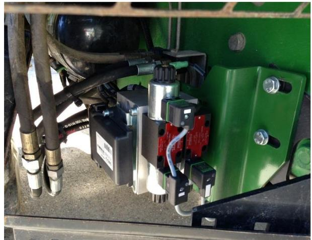
FIGURE 5 MOUNTED MANIFOLD AND STEERING CONTROLLER
