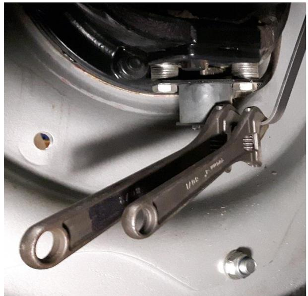
FIGURE 24 BEND THE STRIP WITH THE HELP OF TWO AJUSTABLE WRENCHES.
